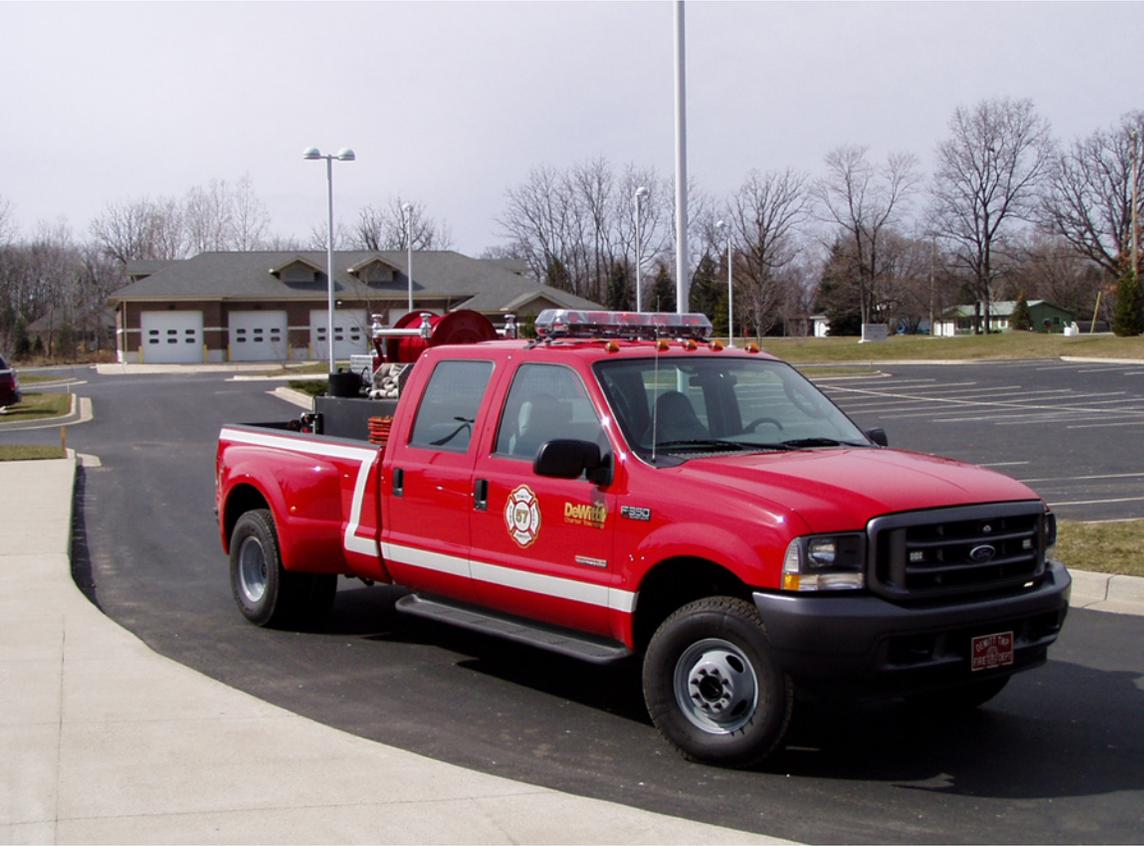
Pictured above is the newest addition to the DeWitt Charter Township Fire Department. This multi-purpose vehicle is used for brush fires and vehicle fires. It is a 2004 Ford F-350 Crew Cab with seating for four. It has a 250 gallon water tank and a 10 gallon foam tank. Brush truck 57 is replacing a 1969 Ford 350.
